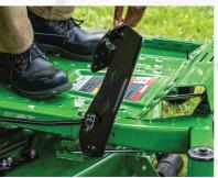
Easily raise and lower your deck with a foot deck lift pedal.
