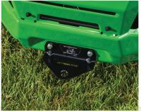
Tow hitches come standard (Z300), with towing capacities up to 250 lbs.
